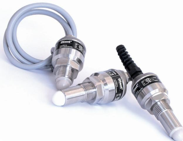
The high-frequency level sensor RFLS-35 is designed for industrial use for limit sensing of the level of liquid and paste-like media. The high-frequency level sensor may be a direct replacement of a vibrating level sensor, or of a capacity level sensor in case of more demanding applications. The media may be electrically conductive or non-conductive with any permittivity. It can be installed in metal or plastic tanks, pipes, filling tanks, sumps, etc.
