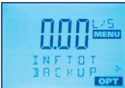
Set the backup of infinite totalizer for storing its value.
