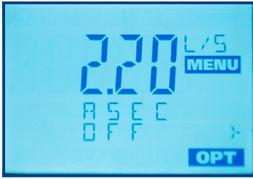
**ASEC (Automatic Systematic Error Compensation)** improves instrument performances. ASEC function works basing on: **Sensor Body Material** and **Pipe Size**. When ASEC is set **OFF**, **Sensor Body Material** and **Pipe Size** options are unavailable in **Calibration Menu**. **WARNING: ASEC** is designed to work **ONLY** in conjunction with F3.00 sensor. Don't activate this function when monitor manage a other sensor.
