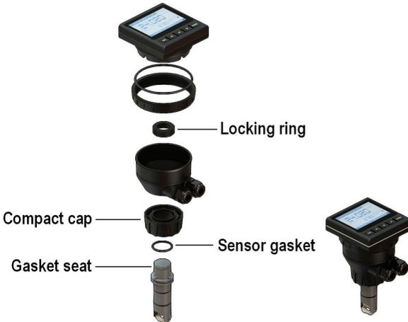
The compact mounting kit (F6.KC1) includes the compact plastic adapter with gasket for IP65 watertight installation, sensor gasket, the compact cap and the locking ring.
