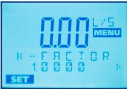
Set the **K-Factor** for the proper conversion of the **frequency** of the flow sensor into a **flow rate**. The **K-factor** is correlated to: **Sensor Model and Actual Internal Diameter** (Pipe Size, Pipe Material, Pipe Standard). Refer to **Flow Sensor Instruction Manual** for the correct value. **K factor range: 000.01 to 99999** (the K-Factor cannot be set to 0)
