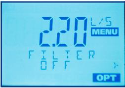
Select the **Filter Level** to dampen fluctuations in measurement.
