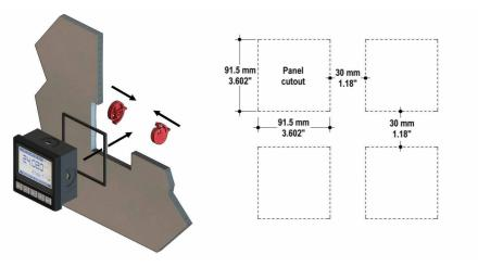
Fix instrument on the panel rotating by hand the fixing snails (M9.SN1).
