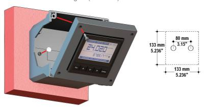
Tighten front screws of box and waterproof connectors of cables, internally mount caps on screw sites to get a IP65 watertight installation.
