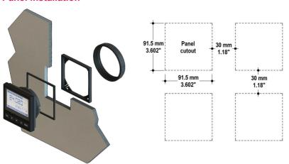
Fix instrument on the panel tightening by hand plastic nut (M9.LN1).
