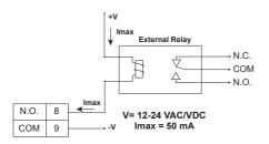
The alarm is off during normal operation and goes ON according to Relay setting.
