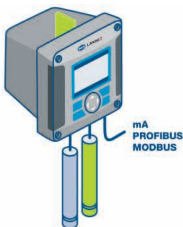
Variant 2: Combined version – one digital SC sensor and one analogue sensor with suitable sensor input card
