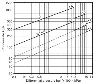
**Note**. Capacities shown are based on discharge at saturation temperature. When discharging sub-cooled condensate the air vent provides extra capacity. Under start-up conditions the thermostatic air
