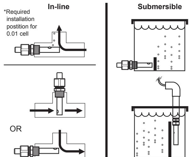
Use caution to avoid air bubbles or sediment trapping inside the electrode cavity.
