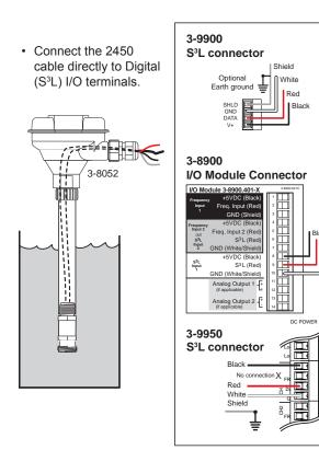
When the 2450 includes a junction box, connect the 2450 terminals to any Digital (S<sup>3</sup>L)
