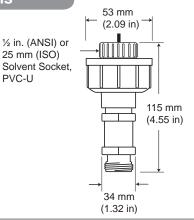
2250 Hydrostatic Level Sensor
