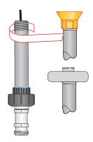
Mount the conduit base onto the adapter and secure the assembly with the locking ring.
