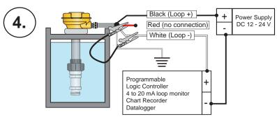
Carefully remove the heat shrink tube that is protecting the red wire.
