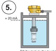
Fill the tank to the level to be represented by 20 mA.
