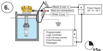
Short the RED and BLACK wires together for 15 seconds.
