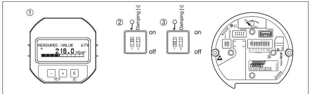
Fig. 26: DIP-switch position "Hardware locking" on the electronic insert
