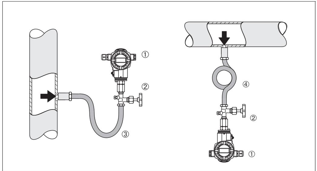
Fig. 6: Measuring arrangement for pressure measurement in steams
