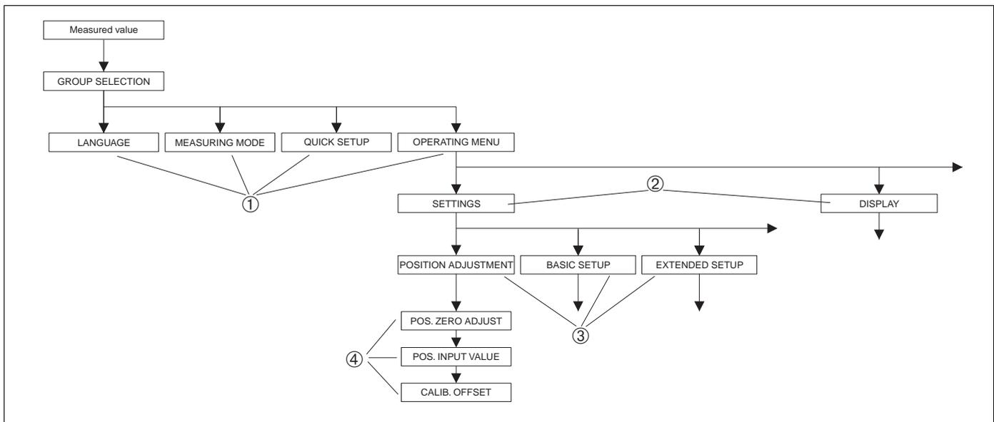
Fig. 25: General structure of the operating menu
