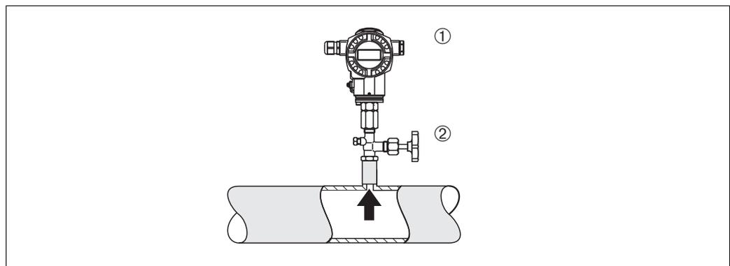
Fig. 5: Measuring arrangement for pressure measurement in gases
