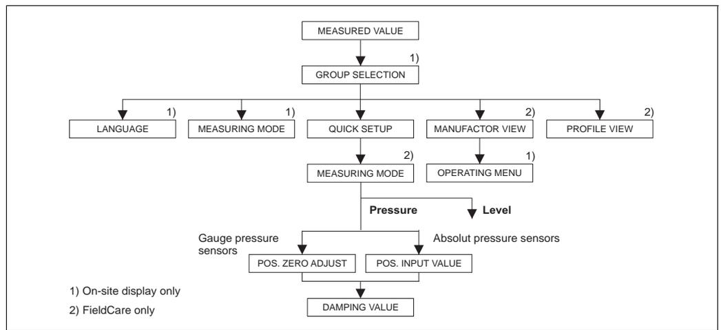
Fig. 27: Quick Setup menu for the "Pressure" measuring mode
