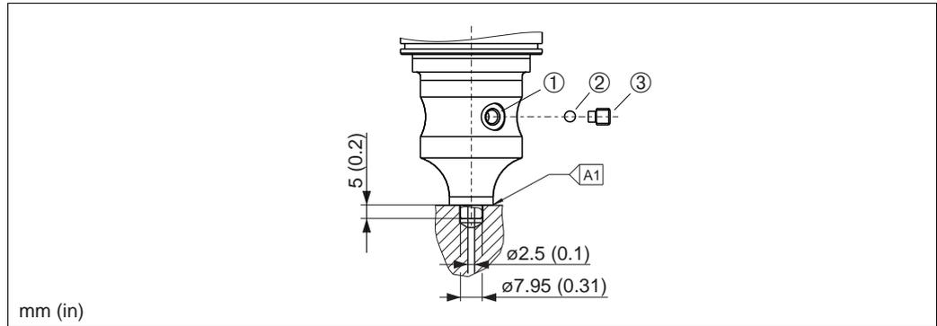
Fig. 14: Version U1: prepared for diaphragm seal mount
