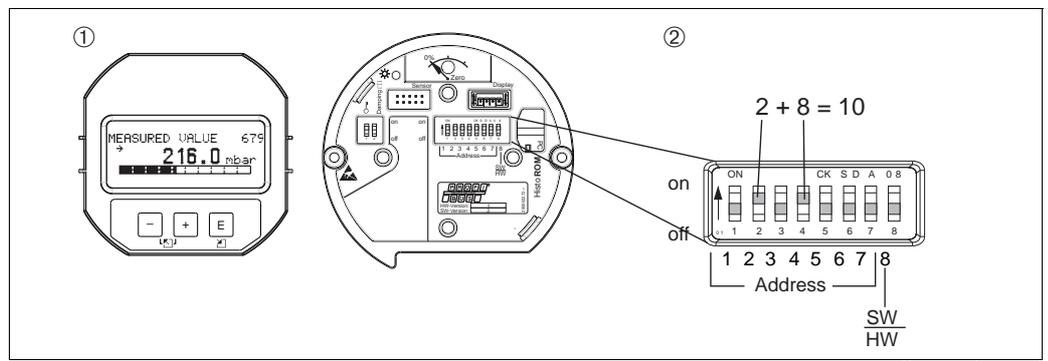
Fig. 22: Configuring the device address using the DIP switches
