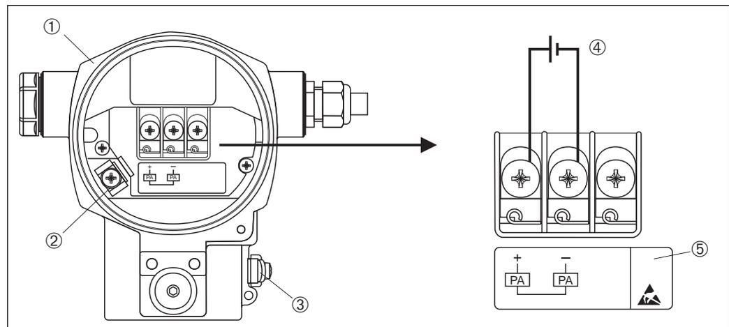
Fig. 17: Electrical connection of PROFIBUS PA
