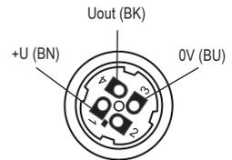
Fig. 6: Inside of the connector socket (variant "C")
