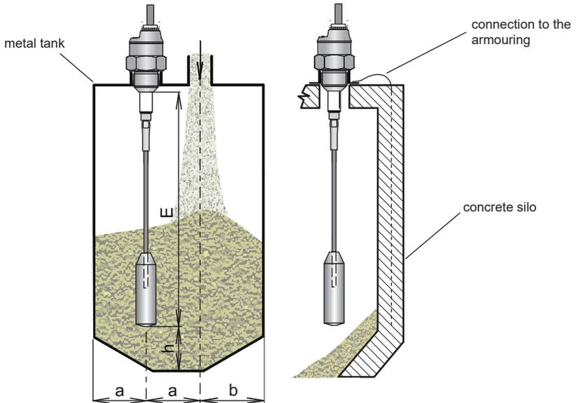
**E** - electrode length [mm] - select so that the end of the electrode would be at least 20 mm under the lowest measured level
