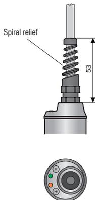
Variant "H" with cable gland for protected hoses - for using in an outdoor area or in area with increased moisture.
