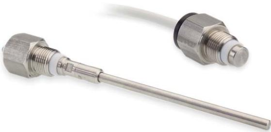
**Conductive probes CNP-18** are designed for direct detection of conductive liquids level (water, water solutions). The process connection is M18x1,5 threaded connection, and electrical by fixed cable or screw connector. The probes are connected to Dinel evaluation unit, type CDSU-522-W, or other types of evaluation units suitable for connection of the conductive sensors.
