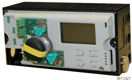
Fig. 7: Open TZIDC with a view of the operating panel
